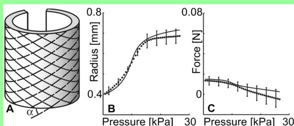
Fig. 2. Comparison of outer radius and axial force (dotted lines) with SEF developed by Holzapfel and Gasser (solid line). Zulliger M.A., Journal of Biomechanics 2004 (37) pp. 990 & 996
