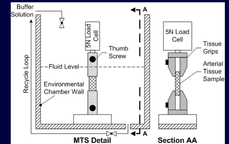
Fig. 2 Detail of material testing apparatus
